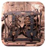
To keep it ticking for many years to come, the clock which is showing signs of wear will soon undergo restorative works. This will involve temporary removal so any congealed oil and grease can be removed, then the pivots will be re-bushed and the clock rebuilt and tested before returning it to the church.
